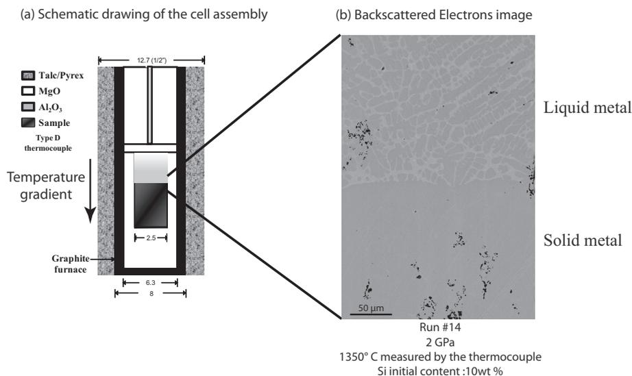
Fig. 1. (a) Schematic drawing of the piston-cylinder 1/2" assembly. (b) Backscattered electron image of a recovered sample showing the coexistence of liquid and solid Fe–Si alloys. The liquid can easily be distinguished from the solid due to its dendritic quench texture. Dark features on the SEM image correspond to small SiO<sub>2</sub> grains crystallizing due to partial oxidation of silicon metal.
